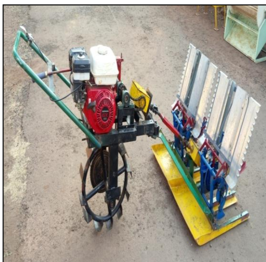
Fig. 1: View of power operated paddy transplanter
